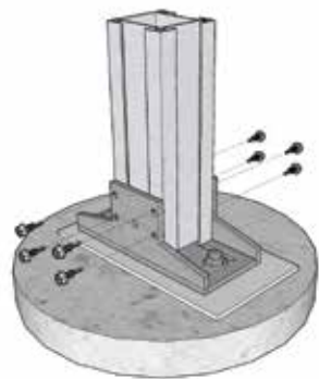
Insert 55mm Profile in bracket (Cut to desired height) secure profile with 8 hex screws
