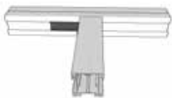
Joist to perimeter joist (Non direct load bearing)
