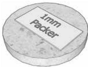
Insulating packer or similar to provide barrier between concrete and aluminium bracket must be used
