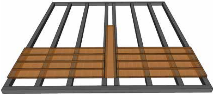
Breakerboard using 1x Additional joists
