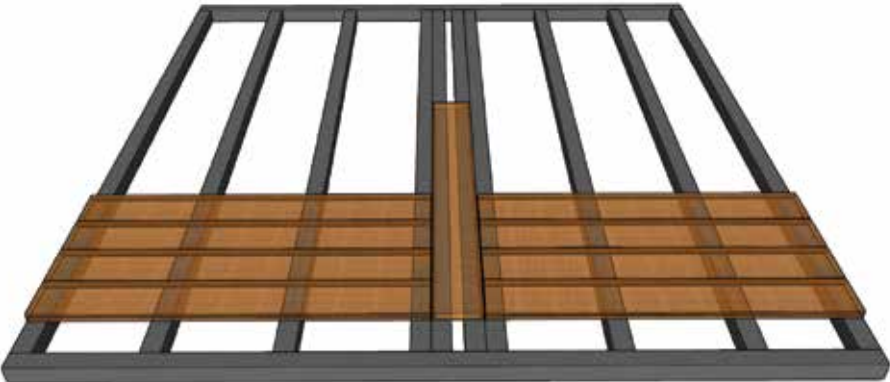
Breakerboard using 2x Additional joists
