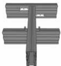
Joist to perimeter joist Non direct load bearing (2 per join)
