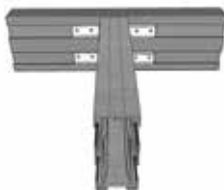
Joist to intergrated bearer Load bearing connection (4 per join)
