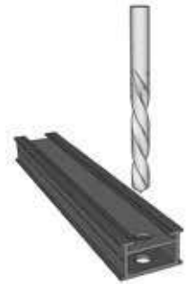
Predrill 28Profile (Max 8mm diameter hole)
