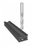
Predrill 28Profile (Max 8mm diameter hole)
